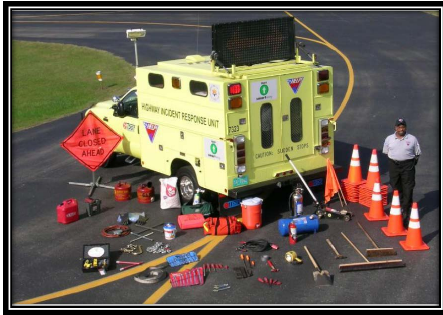
Figure 18: Highway Incident Response Unit with Supplies Displayed
